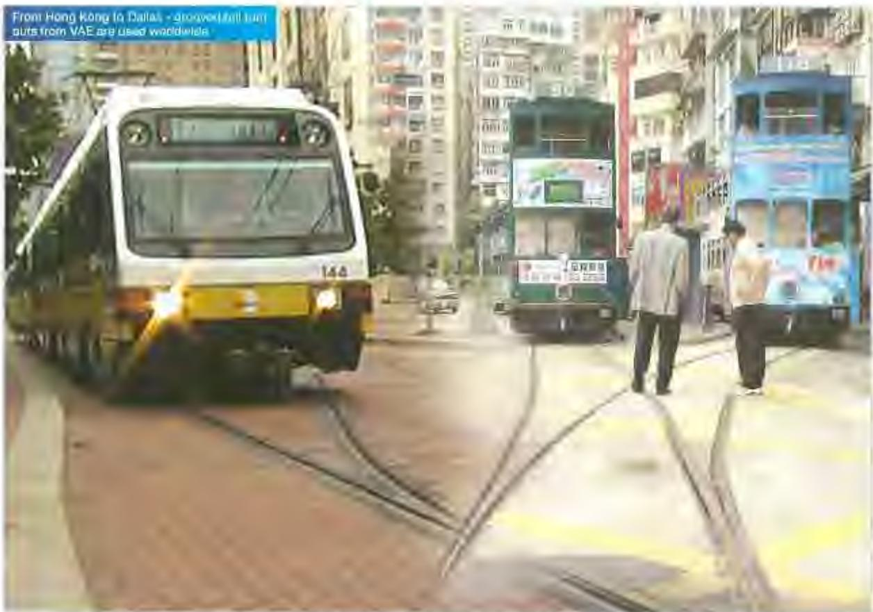
Grooved rail switch devices for light rail / tram systems consist of two sets, connected by tie rods. Standard geometries have radii of 20, 25, 50, 100 and 150 m. Special designs are also possible.
