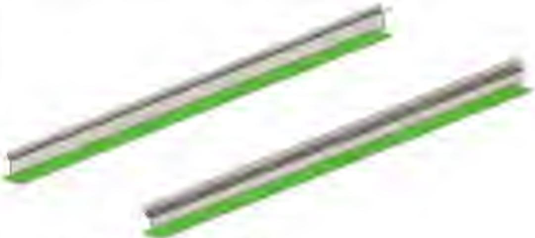
Picture: continuously supported rail
