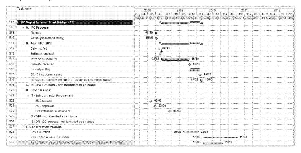
A. **IFC Process:** planned IFC date was **07/10/08**; actual was **10/10/08** i.e. 3 days late; no material delay. We are advised that one drawing was reissued on **13/11/09**. That however was not identified as a material factor delaying commencement; nor was it identified as being critical to construction.
