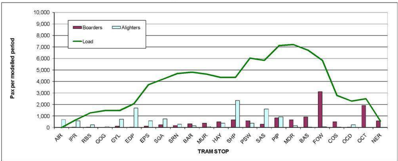
Figure 3.5 – Westbound Boarding and Alighting 2031 AM Peak, Full Phase 1a (Source JRC - June 2011)
