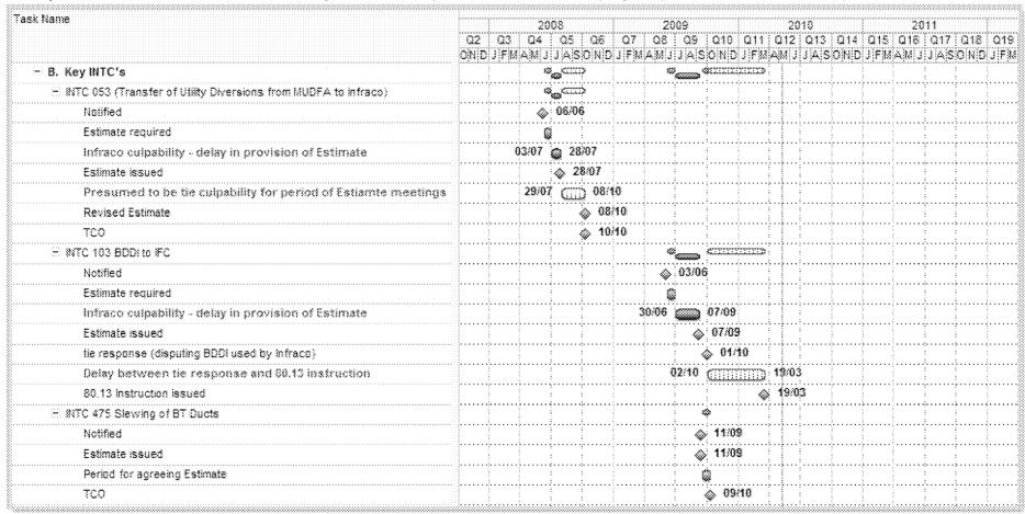
(i) <u>INTC 053 (Transfer of Utility Diversions from MUDFA to Infraco)</u>: we understand that this was a critical delay to commencement of the A8 Underpass. Delay from planned commencement of 28/8/08 to 13/10/08 (i.e. allowing Infraco mobilisation period). **Minimum 5 weeks delay;** tie culpability. Likely be delay of 7 weeks to 13/10/08 (when piling actually started; allowing for mobilisation)
