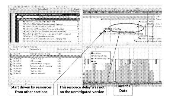
d) To demonstrate the delaying impact of these preferential logic links I have removed them from this section of the programme network and used the computer software to re-scheduled the programme. The result is shown below.
