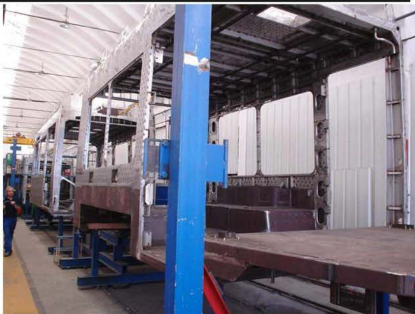
A-4 + B-4 Bodyshells in the measurement jig
