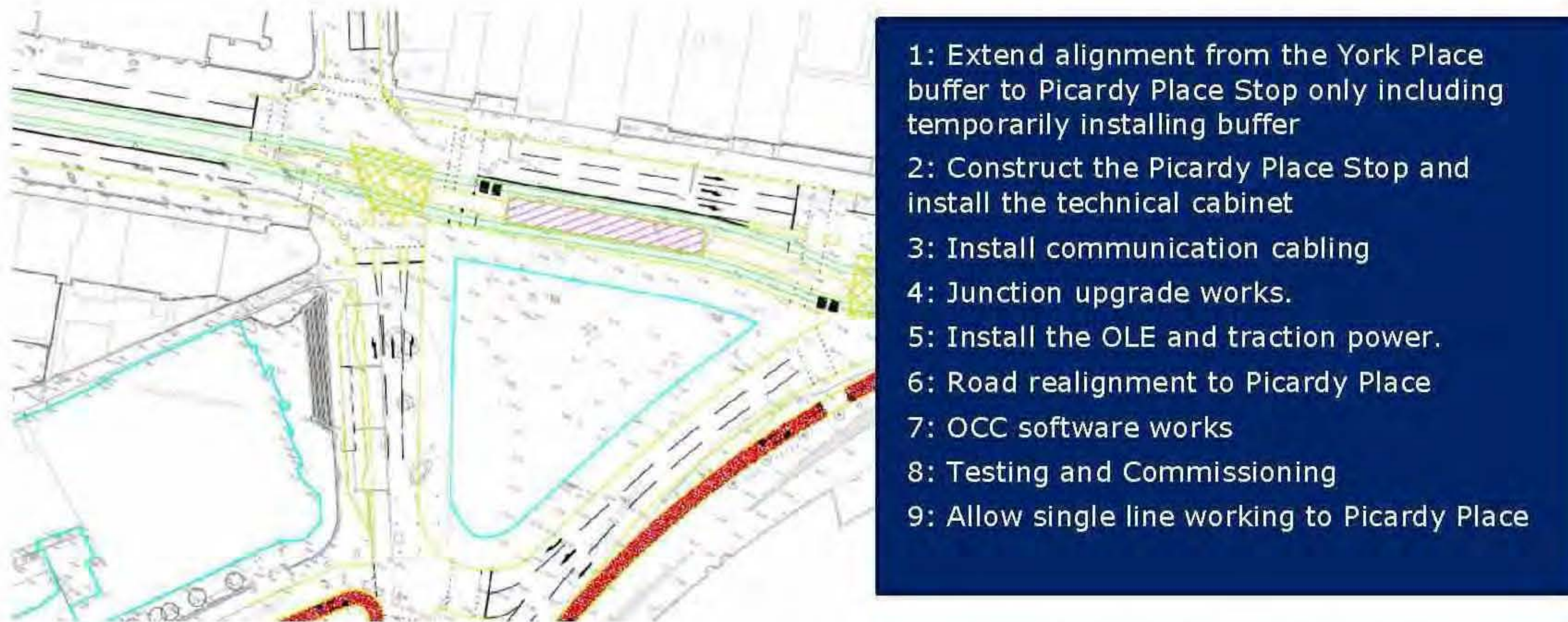
Figure 13: Proposed new tram alignment and Picardy Place junction upgrade works with sequencing
