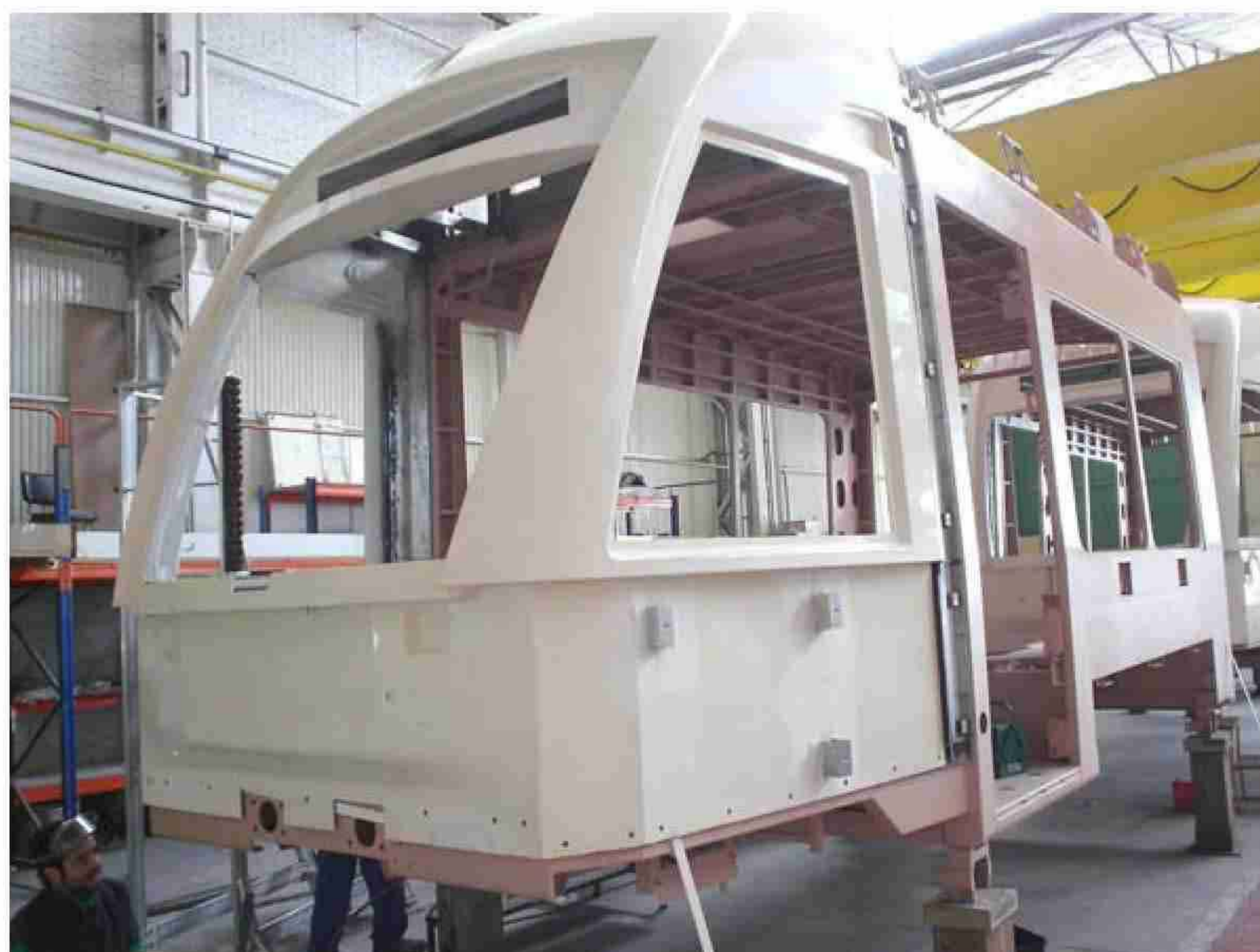
E-1 Front nose assembled
